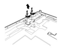
Figure 4-20 Removing the Power Button board
